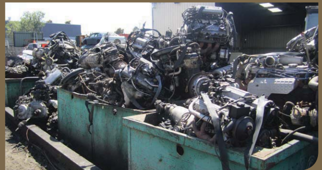
FIGURE 21: MOSTLY COMPLIANT WORKSITE, STORAGE BINS ARE IN A BUNDED AREA BUT BINS ARE TOO FULL AND PARTS ARE STACKED TOO HIGH
