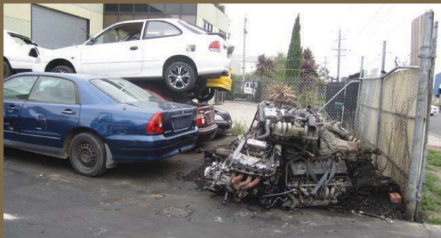
FIGURE 27: COMPLETELY NON-COMPLIANT WORKSITE, ENGINES AND VEHICLES STACKED CLOSE TO PUBLIC ROAD AND MEDIAN STRIP, POSSIBLE RISK TO PEDESTRIAN AND ROAD USERS IF VEHICLE FLUIDS LEAK
