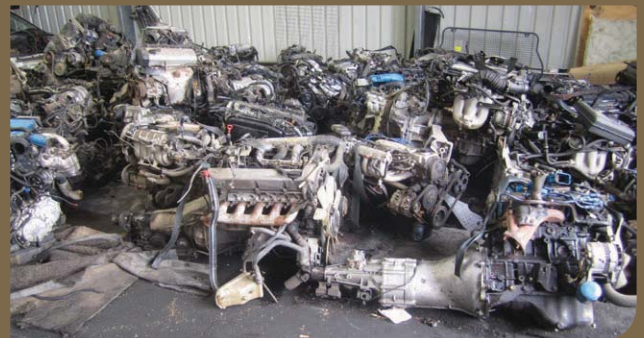
FIGURE 29: COMPLETELY NON-COMPLIANT WORKSITE, ENGINES STORED ON WORKSITE FLOOR, LACK OF BINS OR STORAGE CONTAINERS
