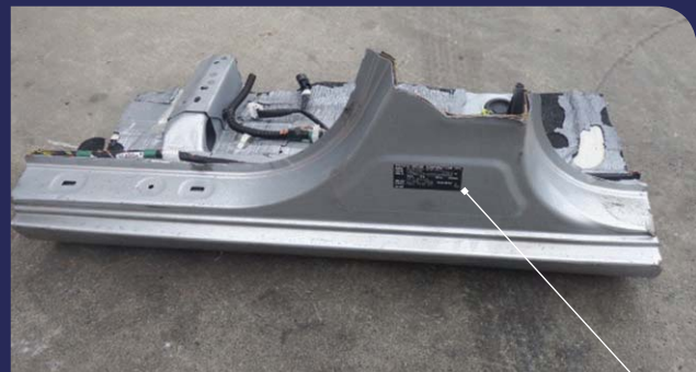
FIGURE 12: SECTION OF SILL AND 'B' PILLAR FROM A STOLEN TOYOTA RAV4, BUILD PLATE ATTACHED
