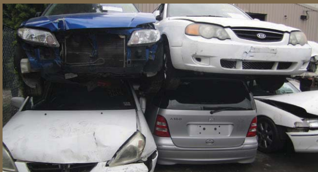
FIGURE 28: COMPLETELY NON-COMPLIANT WORKSITE, VEHICLE BODIES STACKED UNSAFELY
