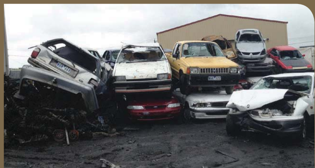
FIGURE 26: SUBSTANTIALLY NON-COMPLIANT WORKSITE, VEHICLE BODIES STACKED UNSAFELY
