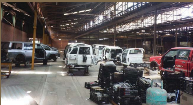
FIGURE 16: SUBSTANTIALLY COMPLIANT WORKSITE, VEHICLES PROCESSED INDOORS ON A SEALED SURFACE
