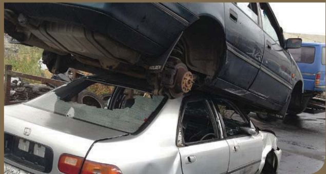
FIGURE 25: SUBSTANTIALLY NON-COMPLIANT WORKSITE, VEHICLE BODIES STACKED UNSAFELY
