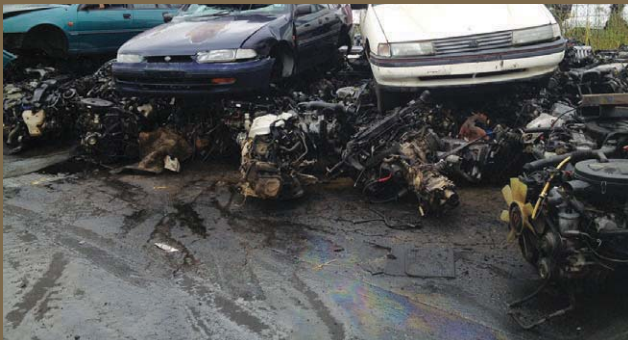
FIGURE 23: SUBSTANTIALLY NON-COMPLIANT WORKSITE, VEHICLE BODIES STACKED ON TOP OF UNSECURED PARTS AND ENGINES WITH FLUIDS ON GROUND
